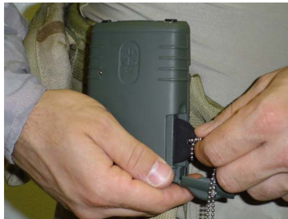
Figure 2-4: WPSM-IC Computational Center (Hub), Showing the Insertion of the Personal Information Carrier (PIC – A Memory Card Containing Medical Records and Personalization Information for the Algorithms). Once the PIC is inserted, the hub will be keyed to an individual and the personal information used to personalize the models and classifiers.
